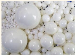
Left: 8YSZ powders and 8YSZ balls for ball milling Right: Slurry degassing thanks to a water Venturi pump
