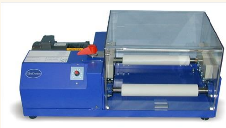
Ball milling equipment for dispersing the powders in aqueous and organic slurries.
