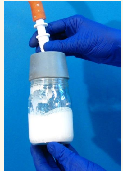
Left: 8YSZ powders and 8YSZ balls for ball milling Right: Slurry degassing thanks to a water Venturi pump
