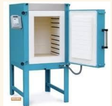
Muffle furnace of 150 liters for cell sintering until 1400°C
